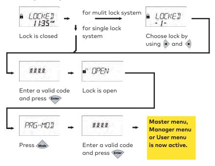
**Note** There are three different Programming modes available in the Axessor series. Enter the Master code, Manager code or User code to access the desired programming level.
