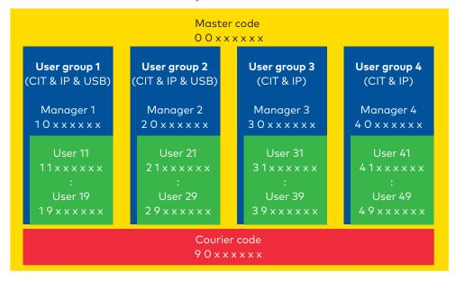
Note The overview shows the code structure of the Axessor series units.
